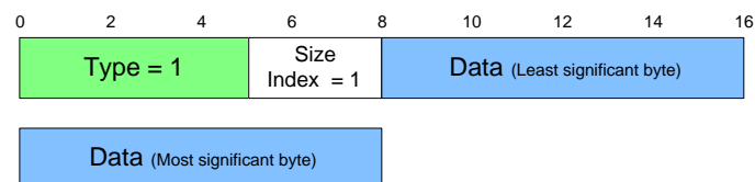
Figure 4.1: Example of a Data Element, containing a 16 bit unsigned int.
