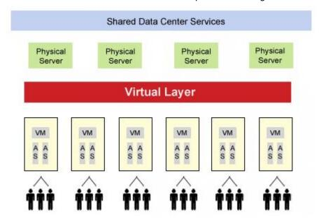
In this simplified representation of a multi-tenant architecture, physical servers share data center resources on the back end. Virtualization is used to create multiple virtual machines (VM) and application spaces (AS) that are independent of physical devices. Each group of customers sees only its own applications. This architecture provides the illusion of a customized computing space while achieving efficiencies through economies of scale due to consolidation.
