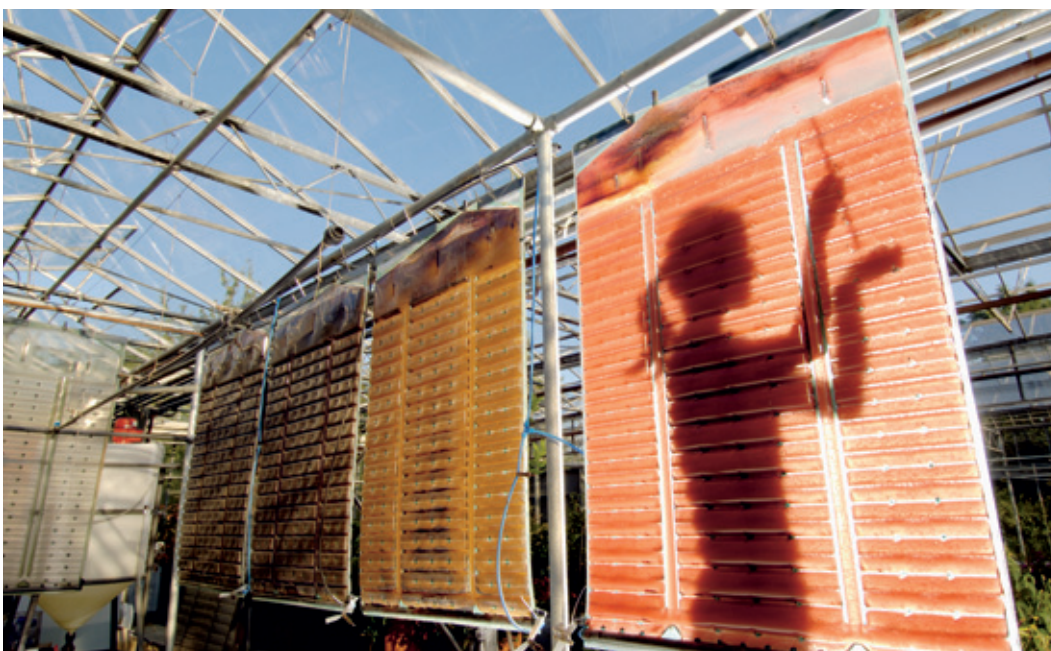
Biostat production plant: Algae produce a valuable red dye for the cosmetics industry.
