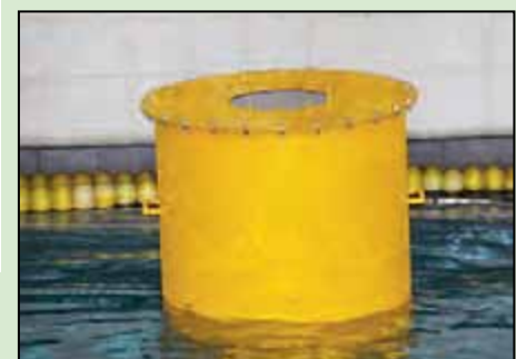
Fig. 2 - Floating OWC 1:35 scale model during preliminary tests.
