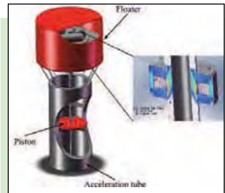
Fig. 1 - Three-dimensional representation of the IPS wave power buoy and electromagnetic brake to simulate the power take-off unit in a 1:35 scale model.
