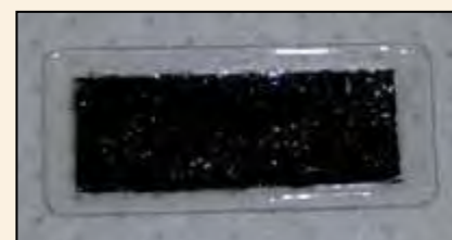
Fig. 3. PDMS membrane with embedded ACNTs.
