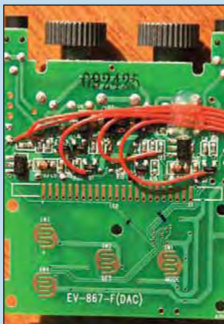
Fig. 1. First FES prototype developed, capable of delivering customized electrical stimuli to one muscle group.
