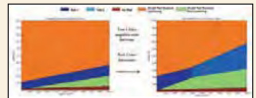
Fig. 4. choice of optimal testing strategy based on minimizing expected value of cost is highly sensitive to individual cost parameters including warranty and scrap cost as well as test costs and error rates.
