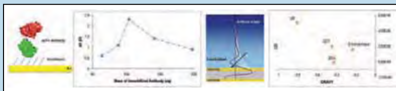
Fig. 3. TSM acoustic sensors are being used to monitor conformational changes and to correlate the protein GRAVY score with acoustic energy losses.
