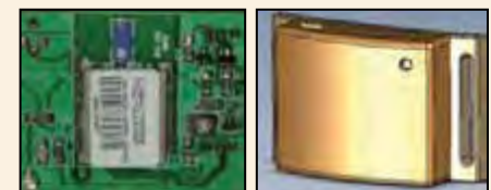
Wireless temperature sensor prototype
