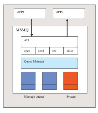
Figure 12. MSMQ Product Architecture. The Queue Manager connects to other Queue Managers in order to communicate between different hosts.
