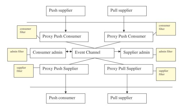
Figure 7. Components in the CORBA Notification Service [GCSO01].
