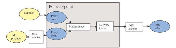
Figure 5. The OpenFusion Notification Service with JMS point-to-point interoperability [Pri01].
