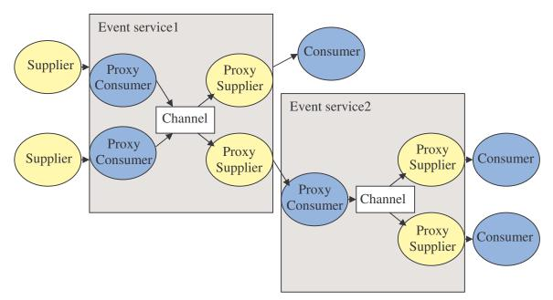
Figure 9. CORBA Notification Service channel federation.
