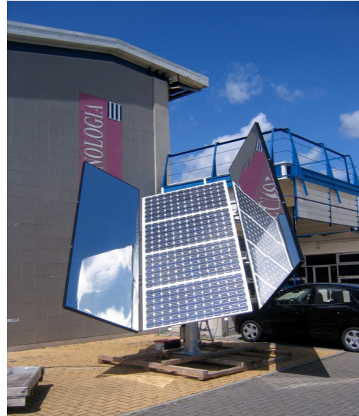
Figure 1: Photograph of DoubleSun solar concentrator in WS Energia laboratory in Portugal (38°41'50"). This system has a peak capacity of 1.0 kWp.
