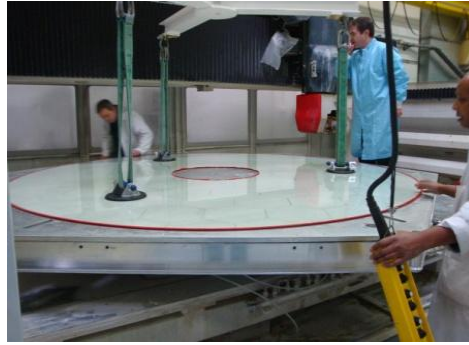
2.6m glass shell, 2 mm thick at SAGEM
