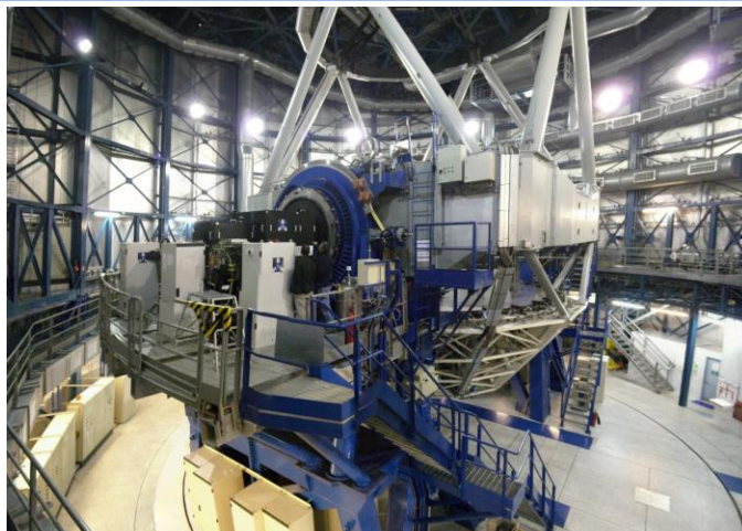
MAD: 2 arcmin FoV, at 2.2 \mu m (K band), using two DMs, a SH WFS (for the Star oriented MCAO reconstruction), and a Multi-Pyramid WFS (for the layer oriented MCAO reconstruction)
