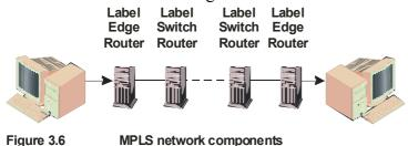
The major difference from a regular IP network is that a Label Edge Router (LER), which is the first and the last router in the network, (figure 3.6) will check the destination and insert an extra header with
