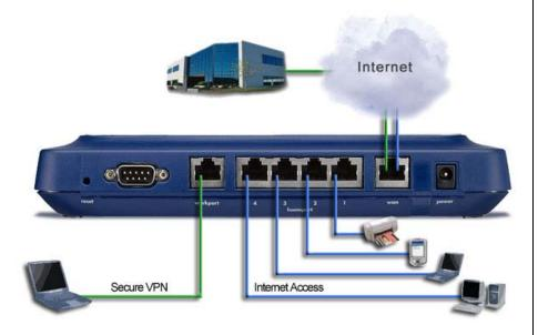
The TELE3 TZX creates two "trusted zones" by creating a firewall between the HomePort™ and the WorkPort™. This additional layer of manageable protection eliminates the risk of unauthorized access through the corporate VPN, while still maintaining connectivity to home network resources.
