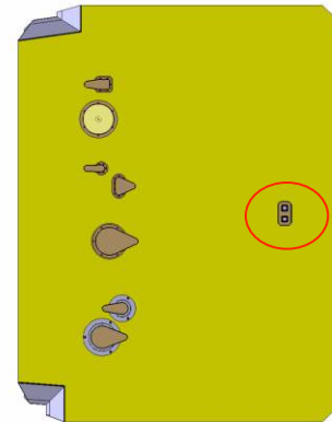
Sun sensors on front face
